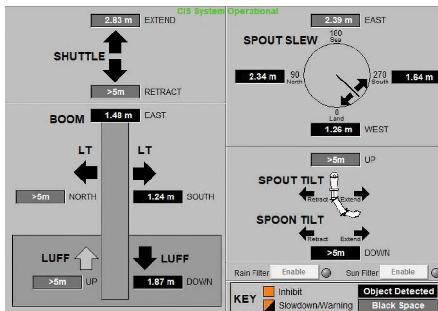
SCADA display showing key separation distances.
