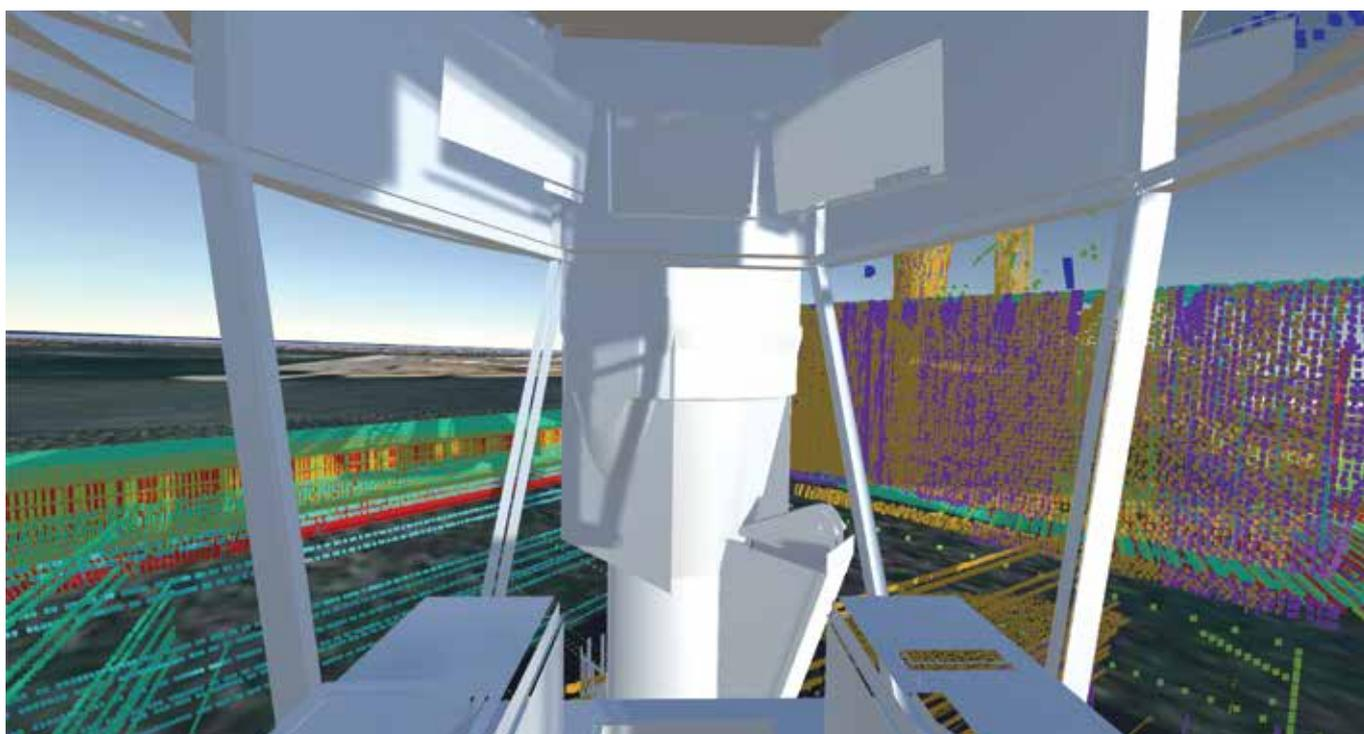
The laser models level of detail and breadth of point of view is evident in the images above. **Top:** Port Kembla Ship loader laser models perspective from under the boom with the spout lowered into the hatch. **Above:** Port Kembla Showing the perspective from the operator's cabin on the boom with the spout lowered into the hatch.
